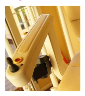
Stair lifts require you to maintain pressure on the controls all the way up and down the stairs. This is most often a lever of some kind at the end of the right arm rest for most models. Most manufacturers allow the installer to move this control to the left arm rest if need be. Be sure to check with your installer to see if moving this control is possible.
